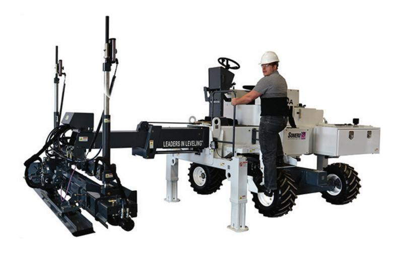
With operator conveniences unmatched in the industry, the **S-10A** was engineered for productivity and convenience. Despite its compact size, the S-10A is highly productive, screeding 200 square feet per pass thanks to its 20' / 6 m telescopic boom and a patented, fully-automated, self-leveling, 10' screed head. Surprisingly lightweight, the S-10A Laser Screed® model can be easily transported.
