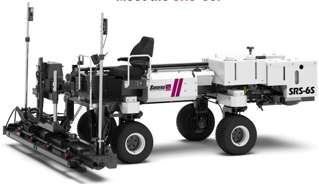
Introducing the Somero SRS-6S Laser Screed® machine - which seamlessly retains the exceptional benefits of its predecessor, the SRS-4, while introducing enhancements that redefine maneuverability and a 12' head that increases production.
